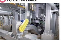
the Fly Ash Circulator, and any unreacted slaked lime which used to be discarded — is reused. This effectively reduces the amount of slaked lime consumed while also reducing the amount of fly ash generated.
