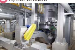
the Fly Ash Circulator, and any unreacted slaked lime which used to be discarded - is reused. This effectively reduces the amount of slaked lime consumed while also reducing the amount of fly ash generated.
